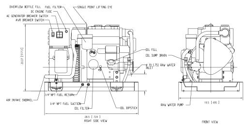
M673L3 Overall Dimensions L x W x H: 28.5 x 19.5 x 20.4 inch (724 x 495 x 517 mm) Sound Enclosure Dimensions L x W x H: 28.5 x 19.5 x 20.8 inch (724 x 495 x 528 mm) Sound Enclosure Weight: 44 lbs (20 kg)
